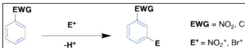
**Scheme 2.** EWGs reduce ring reactivity and steer substitution to the meta position by destabilising the ortho/para arenium ion intermediates.
