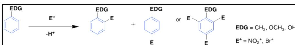
**Scheme 1.** EDGs enhance reactivity and direct substitution to ortho/para or both ortho and para positions by stabilising the arenium ion through resonance delocalisation.
