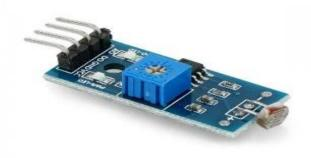
This light sensor module is predicated on a GL5528 photodetector to discover the mild intensity in the environment. Because the resistance of the sensor modifications with the amount of light it's far uncovered
