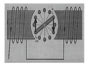
A large percentage of AC motors are induction motors. This implies that there is no current supplied to the rotating coils (rotor windings). These coils are closed loops which have large currents induced in them. Three-phase currents flowing in the stator windings leads establish a rotating magnetic field in the air gap. This magnetic field continuously pulsates across the air gap and into the rotor. This is a single phase representation of windings and current flow
