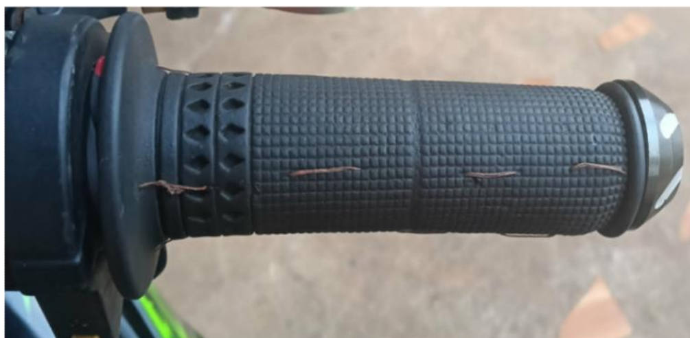
Fig. 2 Electrocutor in the handle grip
